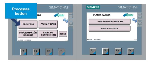
• Timers (Temporizadores) button: users may change the times that they are able to access (for example, the sand cleaning time or the blower operation time) on the 4 configuration screens. These are set up by the manufacturer and should not be touched unless necessary.
